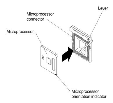
**Note:** Do not use excessive force when pressing the microprocessor into the connector.
